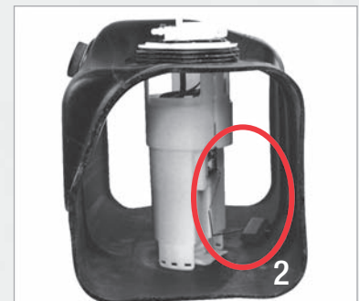
Properly positioned fuel pump module assembly
