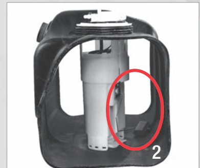
Properly positioned fuel pump module assembly
