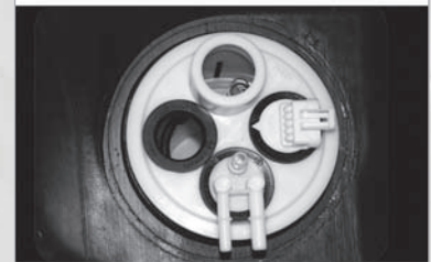
Properly positioned fuel pump module assembly
